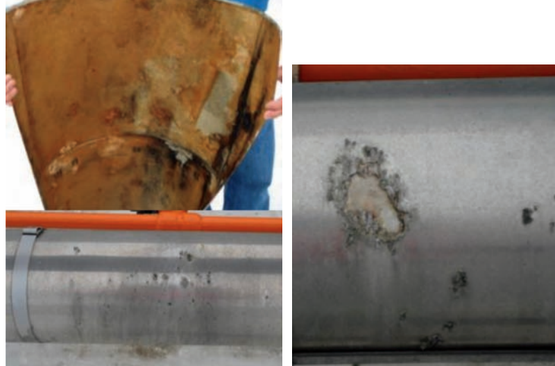
Figure 6 – Pictures of real-world interior surface metal jacket corrosion
